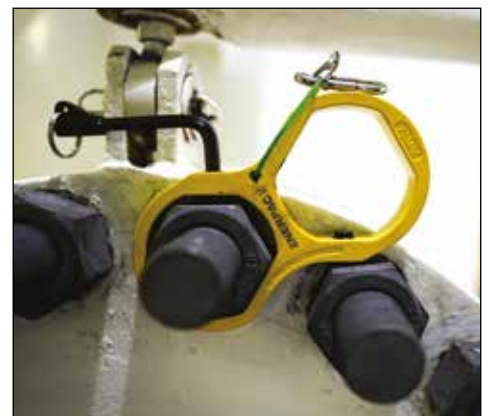
▼ Enerpac Back-Up Spanners to be used to stop back nut from turning during make up or break out.
