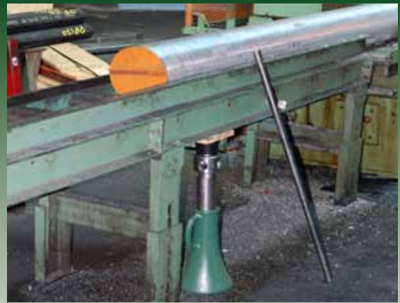
Simplex screw jacks are used to adjust the height of this roller fixture. "We use this fixture during the cutting of long pieces of stock."
