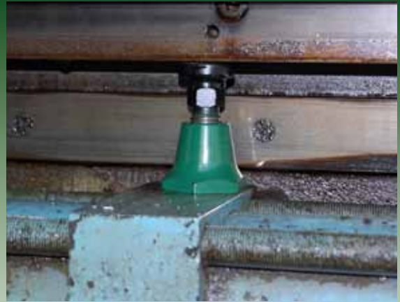
The S3A, with its low profile and small footprint was the perfect solution to level the bed of this milling machine.
